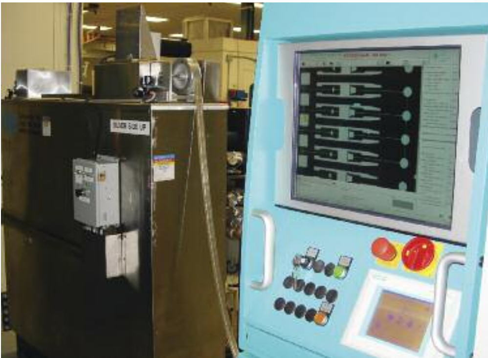
Micro Stamping recently invested in a new high-speed Bruderer press with an integrated inline inspection system (shown here). The system inspects lead-frame stampings at 1200 strokes/min., 12-out per stroke.
