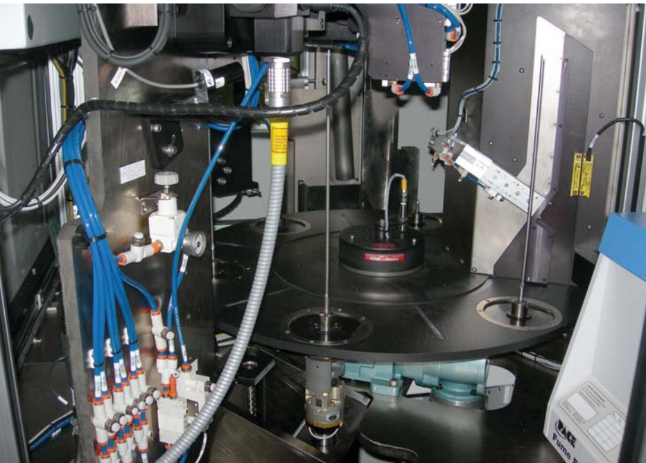
An automated rotary table feeds the laser seam-welding machine.
